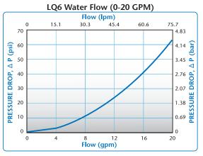
This graph is intended to give you a general idea of the performance capabilities of each product line. Contact CPC for flow of a particular coupling combination
